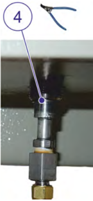
Figure 10.6: Remove snap rings of coolant connections
