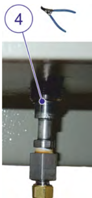
Figure 10.26: Fasten snap rings of coolant connections
