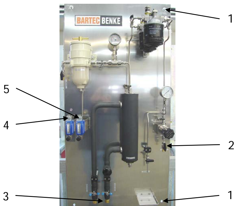
Fig. 7.1: Sample conditioning system (example)
