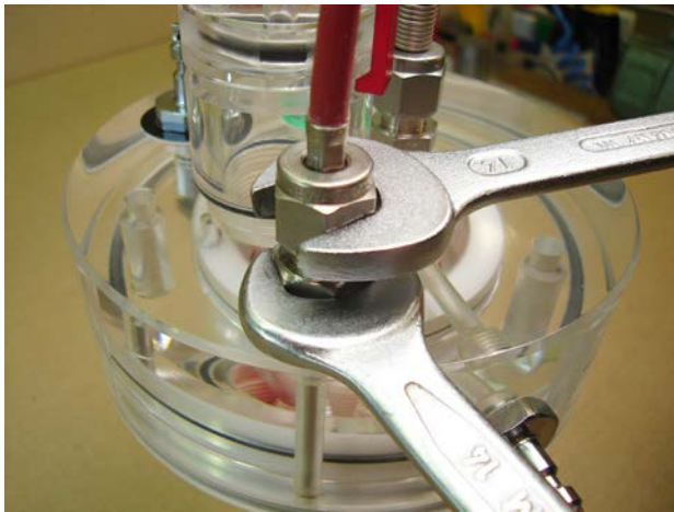
Fig. 10.19: Tightening screw connections
